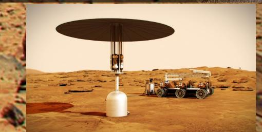
NASA STMD is developing Fission Surface Power (FSP) for Moon and Mars
